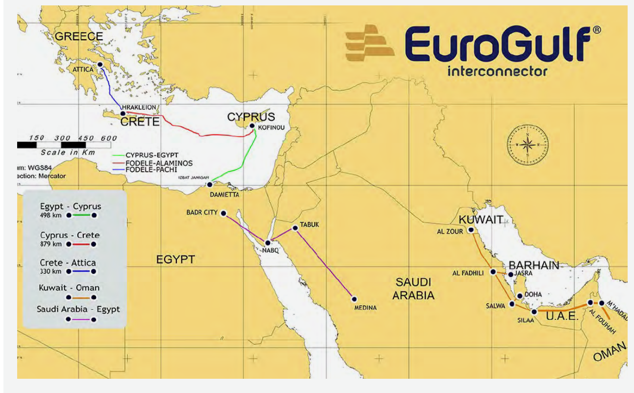
Figure 98: The EuroGulf interconnector's route and its connections through Egypt, Cyprus and Greece to the European Network
