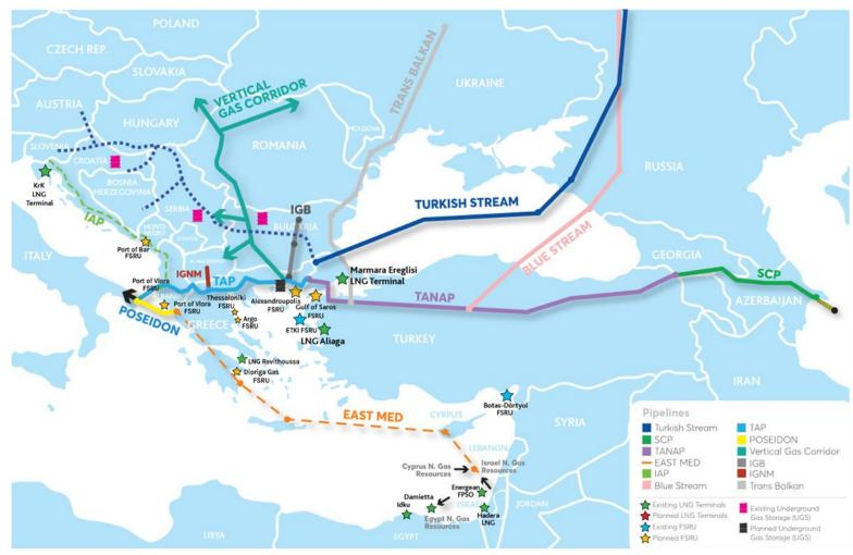
Note: The TANAP, TAP, IGB and Turk Stream have been completed, while BRUA is still under construction. The IAP, the IGI Poseidon in connection with East Med pipeline and the Vertical Corridor and the IGNM are still in the study phase. Blue Stream and Trans Balkan are existing pipelines.
