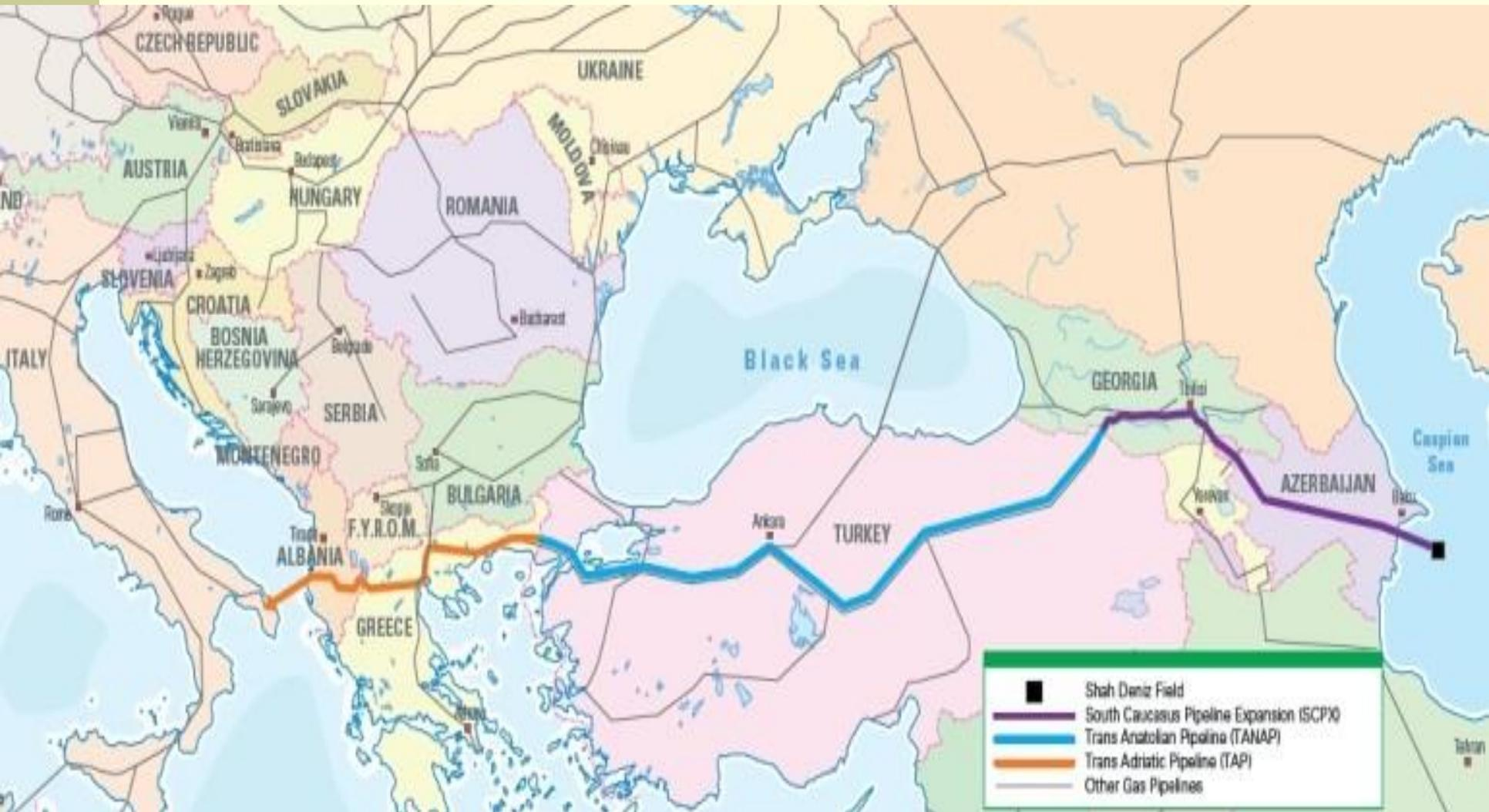
TANAP (60 BCM/y planned capacity) is the central and longest section of the Southern Gas Corridor (SGC) connecting the giant Shah Deniz gas field in Azerbaijan to Europe via the South Caucasus Pipeline (SCP), TANAP & the Trans Adriatic Pipeline (TAP).
