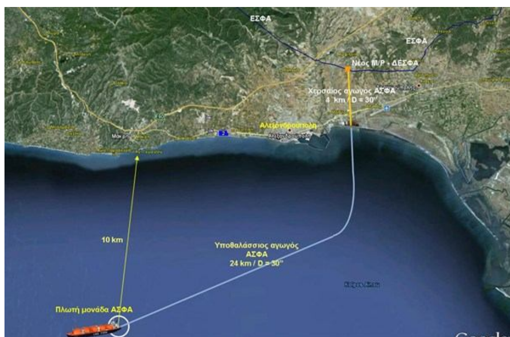
Figure 32: The independent Natural Gas System in Alexandroupolis (Source: Gastrade)
