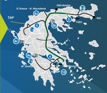
Phase 1: Utilisation of the new system with NG Phase 2: Utilization of the new system for pure H2\* 100% H2 Ready Pipeline: 600 km
