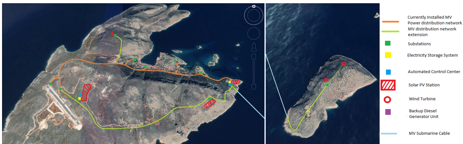
Figure E7: The new integrated RES-Electricity Storage System at the proposed installation sites and the geographical map of the island's micro-grid loop
