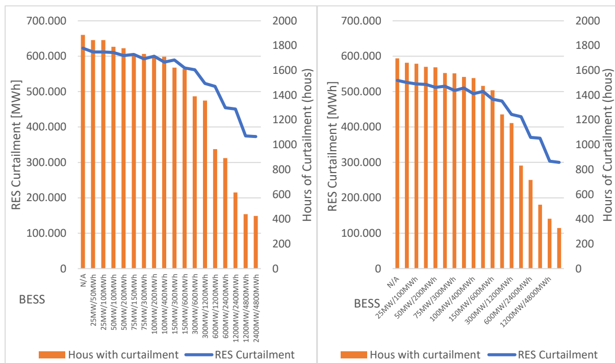
Figure E5 Estimation of curtailment of RES (MWh) and annual accumulated time (hours) of RES's curtailment for scenarios (a) HR30 and (b) HDHR30 for the integration of various BESS in Crete.
