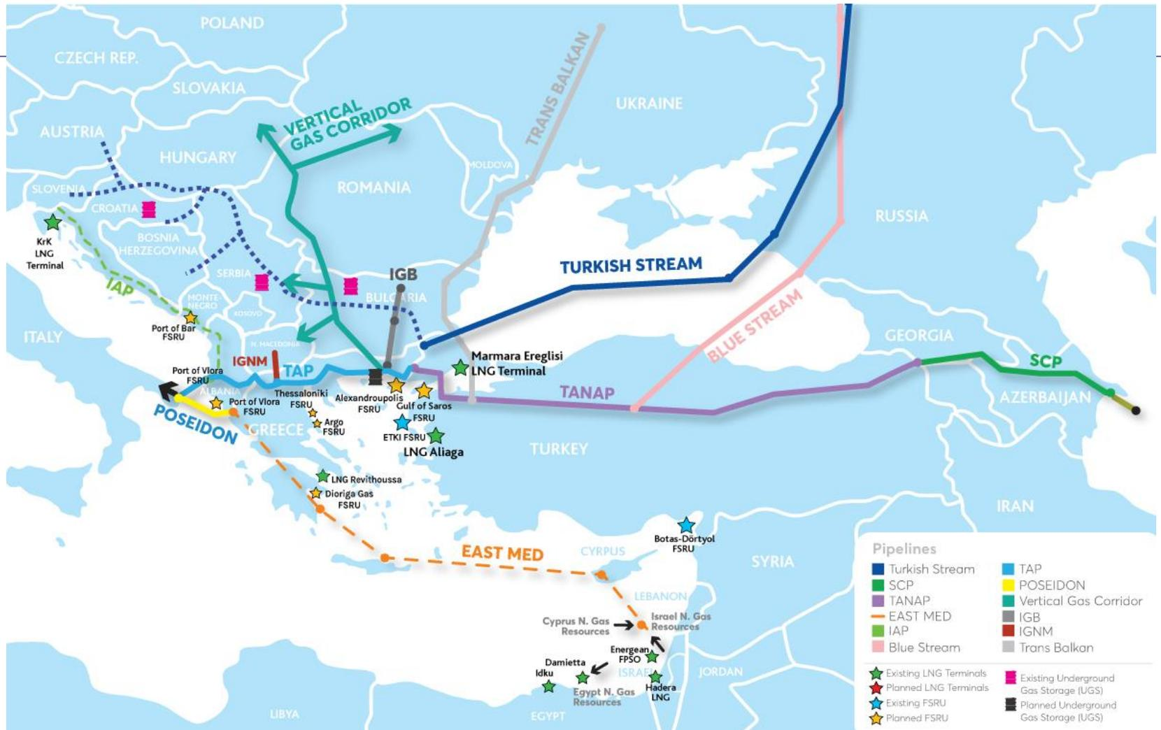
**Note:** The TANAP, TAP, IGB and Turk Stream have been completed, while BRUA is still under construction. The IAP, the IGI Poseidon in connection with East Med pipeline and the Vertical Corridor and the IGIM are still in the study phase. Blue Stream and Trans Balkan are existing pipelines.
