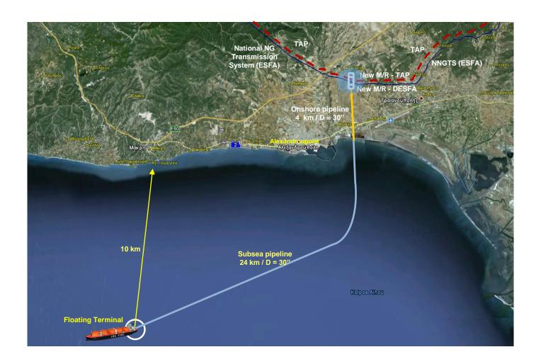
The Project comprises the FSRU and the pipeline system (subsea and onshore sections)
