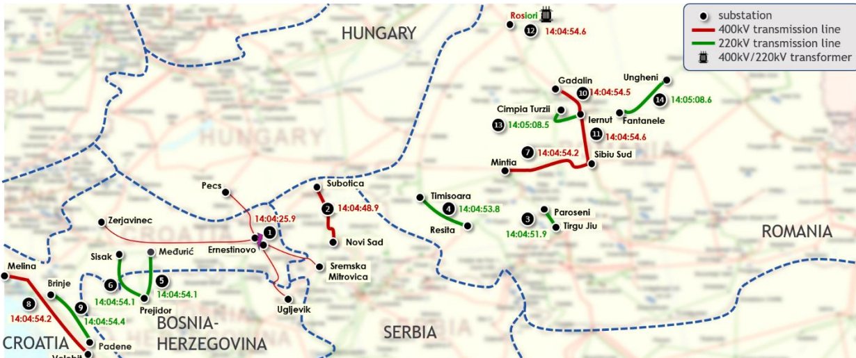
Figure 2 - Tripping of additional transmission network elements after the decoupling of two busbars in Ernestinovo
