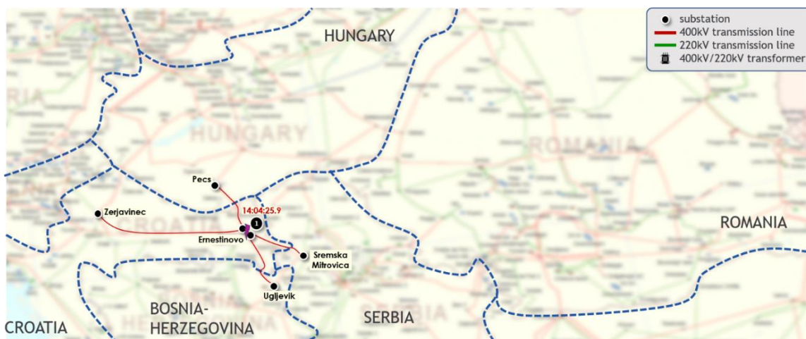
Figure 1 - Decoupling of two busbars in Ernestinovo
