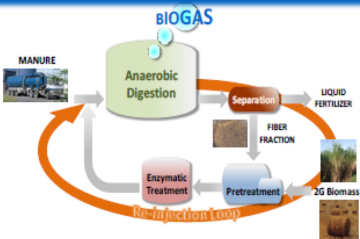
Figure 1 A) Schematic drawing of the Re-Injection Loop concept. B) Drawing of lignin, cellulose and hemicellulose in plants
