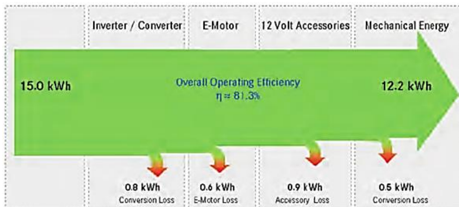
Figure 1 EV Operating Energy Flow and Efficiency Diagram (Source: Abdul-Hat et al.)
