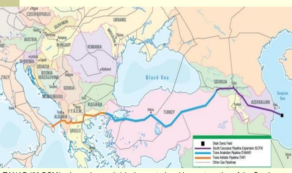
TANAP (60 BCM/y planned capacity) is the central and longest section of the Southern Gas Corridor (SGC) connecting the giant Shah Deniz gas field in Azerbaijan to Europe via the South Caucasus Pipeline (SCP), TANAP & the Trans Adriatic Pipeline (TAP).
