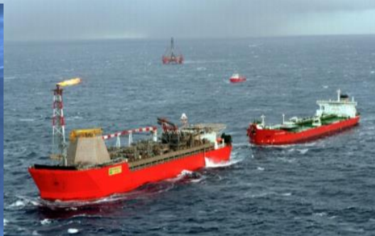
FPSO for condensate storage , pipeline export for gas
