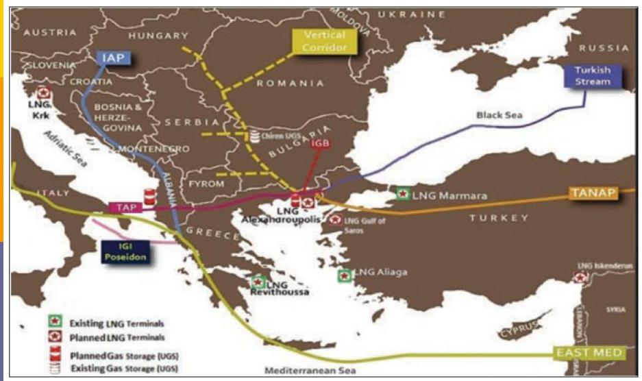
NB.: The TANAP and TAP gas pipelines as well as Turkish Stream are under construction, with IGB at an advanced planning stage with FID already taken. The IAP, the IGI Poseidon in connection with East Med pipeline and the Vertical Corridor are still in the study phase.
